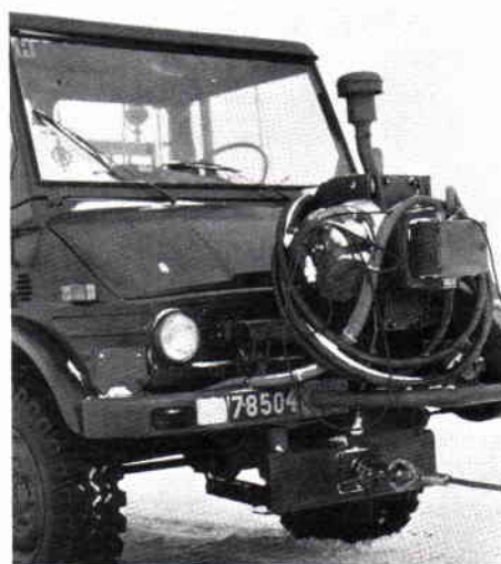
Unimogs okonventionella startgenerator.
